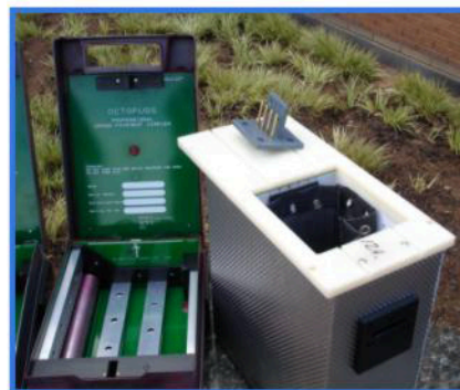
TYPICAL CIT APPLICATION SHOWING DYE DISCHARGE TUBES
